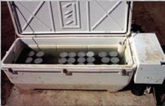
An example of proper field curing methods includes the use of a temperature controlled curing box
