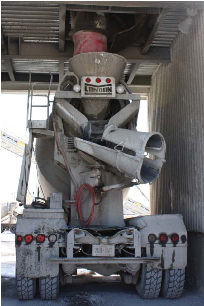
FIGURE 12.1: Concrete truck loading at plant
