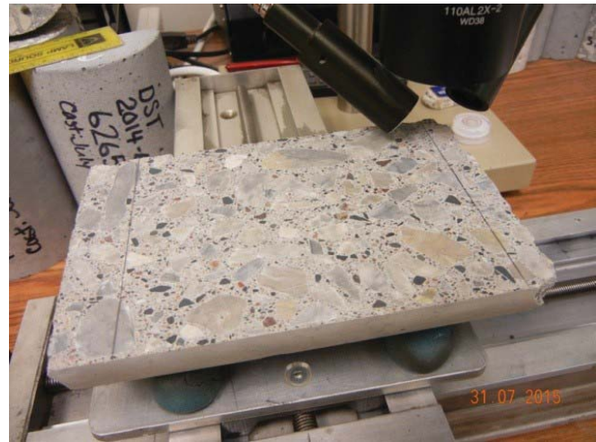
Figure 16.6: Hardened air void test sample Provided by exp Services
