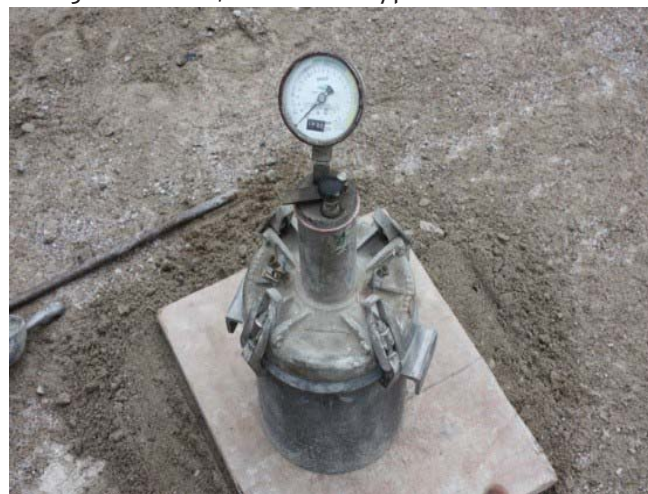
Figure 16.3: Concrete air content test Provided by Concrete Ontario
