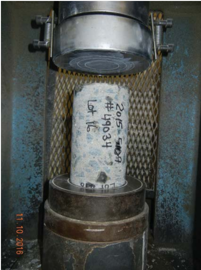
Figure 16.5: Concrete core compression test Provided by exp Services
