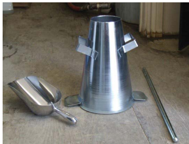
Figure 16.2: Concrete slump test (cone) apparatus Provided by Concrete Ontario
