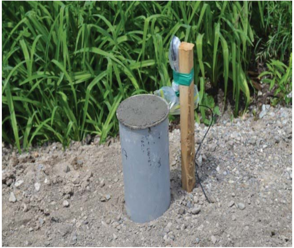
Figure 16.4: Concrete cylinder and maturity monitoring gauge to determine real-time strengths insitu (provided by Concrete Ontario)
