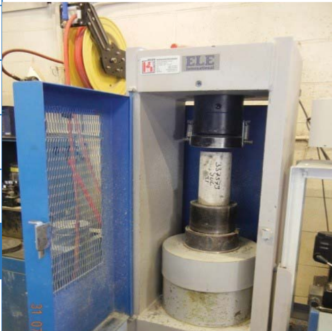
Figure 16.1: Concrete compression test (provided by exp Services).
